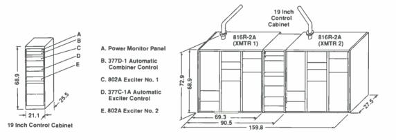
Typical Set-up: 40 kW FM Transmitters
