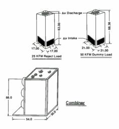
Combiner & Transmitter Dummy Load Configurations for 50,55 kW FM Transmitters
